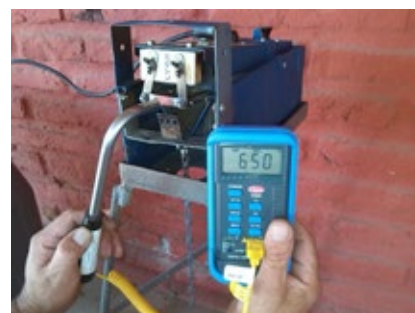
Pyrometer indicating proper blade temperature of 650°C.
